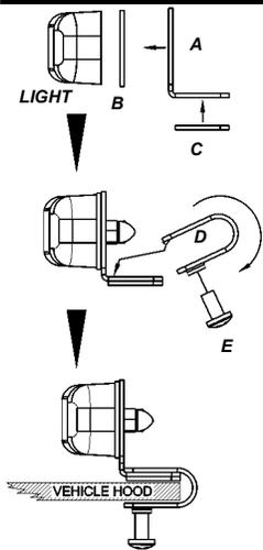
1. Review the diagram on the front page and mount the light to the L-bracket (A) with the gasket (B).
