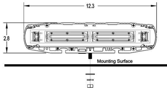
Mount the light through a 11/32" hole using the single bolt on the bottom of the light. Secure it with a flat washer, split washer, and nut.
