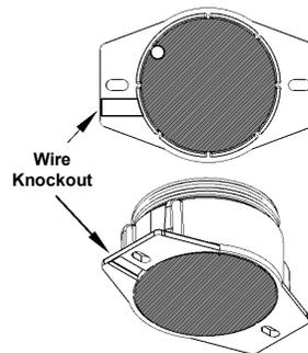
6. Place the light on the mounting surface, routing the wires through the grommet if necessary. Align the outer holes of the base with the holes in the mounting surface, install the screws and nuts, and tighten until snug.
