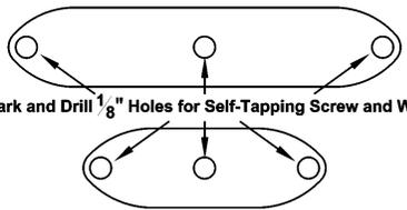
Mark and Drill  $\frac{1}{8}$ " Holes for Self-Tapping Screw and Wires
