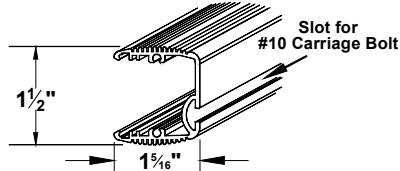
**Please note that the mounting slot must be closer to the lower edge of the light when you mount it to allow for proper draining through the weep holes.
