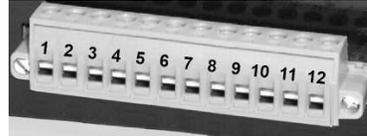
**Park/Kill Feature** - If you would like the siren to automatically disengage when the vehicle door is opened or when the vehicle is placed into park, connect terminal 12 of the green connector to the dome light, added door switch, or added park switch. Review the wiring diagram on the page 2 and ensure that you have the **PK Polarity** DIP switch set for the correct polarity (see next page).
