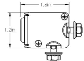
We also include two L-Brackets to facilitate mounting. These are optional and do not need to be used.
