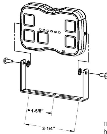
A U-bracket (P/N 274-SB44-U) is included for mounting.
